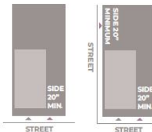
This diagram illustrates the twenty foot minimum requirement for building a side yard ADU on both an infill lot (left) and a corner lot (right).
