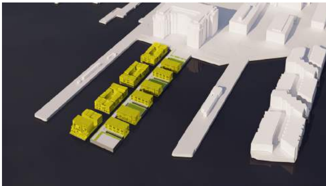
PHASE THIRTEEN - WESTERLY BARGE/VESSEL PLATFORMS ARE FLOATED INTO PLACE
