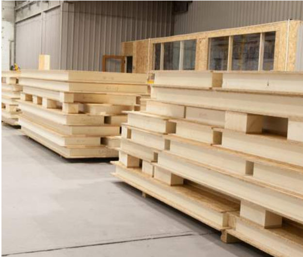
SIPS panels for "The Chichester"
