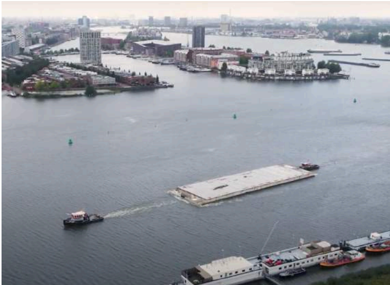
Large Concrete Hull - ready to receive accommodation at destination
