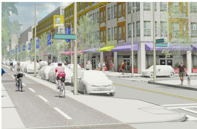
Figure 60. Conceptual drawing of potential "Complete Streets" improvements for Washington Street, including landscaping, protected bicycle accommodations, and improved sidewalks
