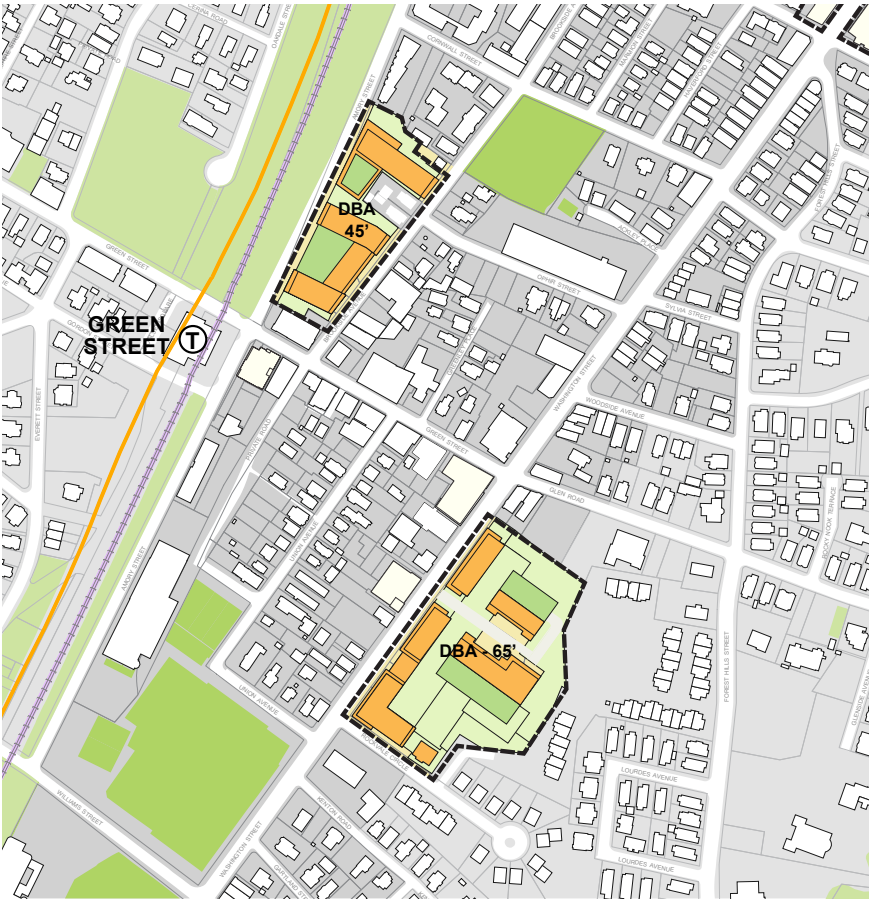
Figure 88. Conceptual plan drawing to provide details of the development scenarios in the Green Street focus area, with height zones
