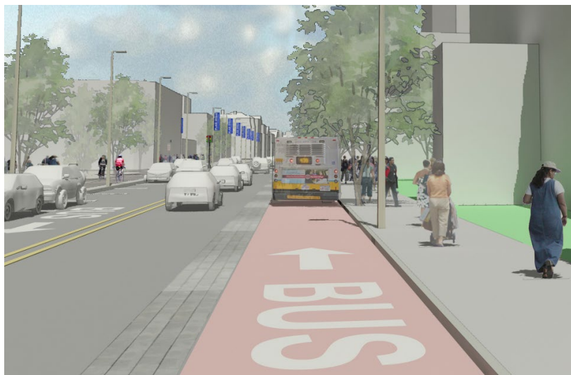
Figure 59. Conceptual drawing of potential "Complete Streets" improvements for Columbus Avenue, including landscaping, bus rapid transit (BRT) elements, protected bicycle accommodations, and improved sidewalks
