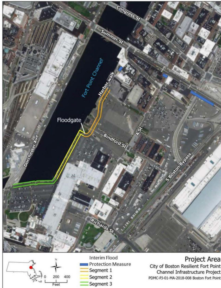
Figure D-3. Components of the Proposed Action including flood control Segments 1, 2, and 3 and interim flood control measures.
