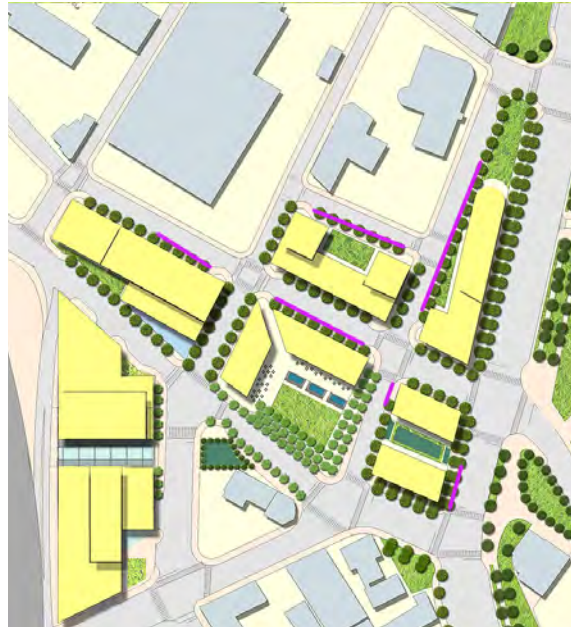
Recommended locations for loading areas and handicapped accessible and pick-up/drop-off parking for building residents is shown in purple on the plan above. Parking and loading for Parcel 1 can be handled internally in the ground floor of the garage.
