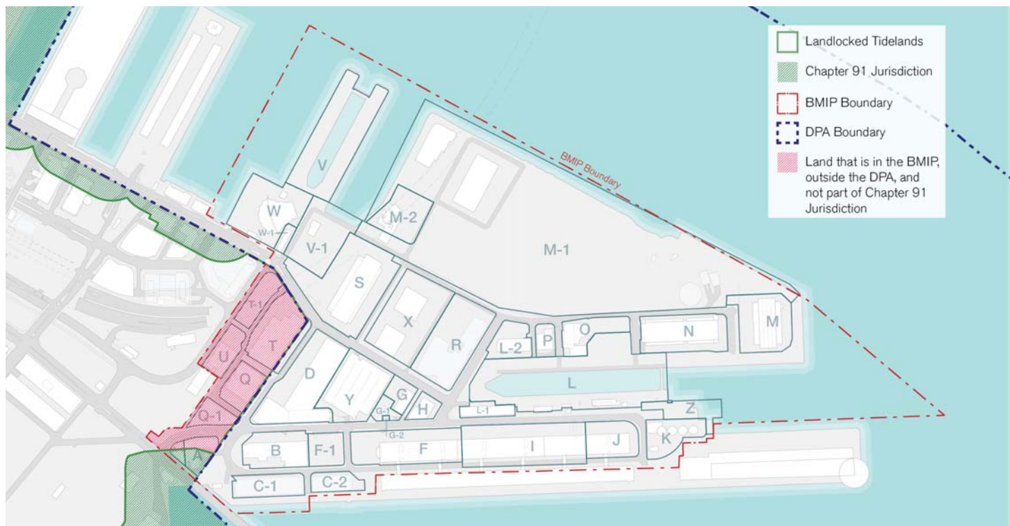
The diagram above highlights those parcels within the RLFMP that are neither in the DPA or within Chapter 91 jurisdictional boundaries. The only regulatory constraints for these parcels is local zoning, which is currently Industrial and is limited to an FAR of 2.
