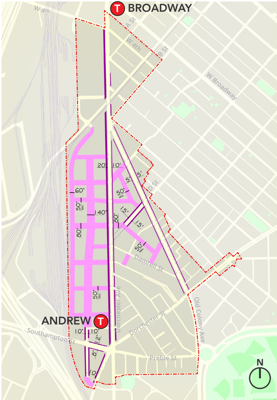
Figure 151. Conceptual diagram of property line setback requirements for creation of R.O.W.s. Exact location and widths of R.O.W.s to be determined by a future transportation study
