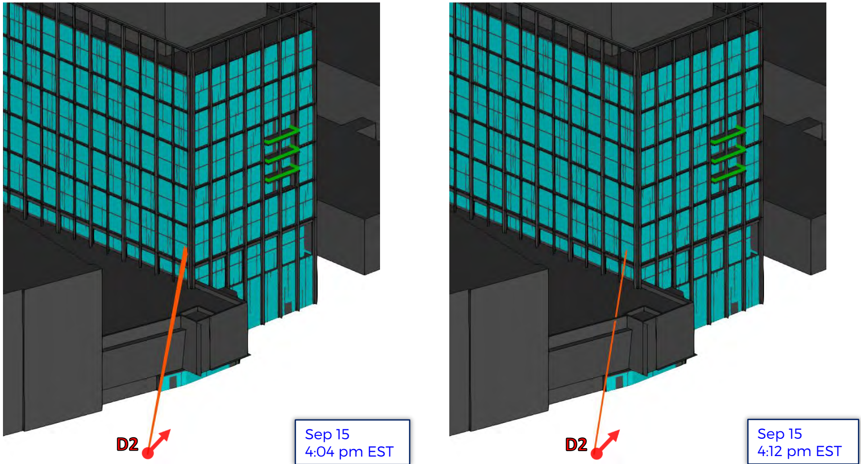
Figure 10: Illustration of reflections with high visual impacts on receptor D2 on September 15. (Some surrounding buildings removed for clarity.)
