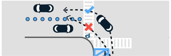
A row of bollards installed on the yellow centerline discourages drivers from cutting turns at higher speeds.
