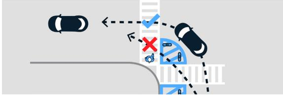
A slow turn wedge is a combination of pavement markings, flexible bollards, and rubber or plastic curbs or bumps. They slow turning drivers to safer speeds.
