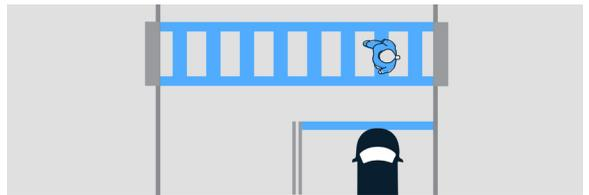
“Ladder” style crosswalks, with thick white bars and parallel lines, are the most visible type of crosswalk marking. High-visibility crosswalks help improve pedestrian visibility and safety. They also help to clarify where pedestrians should cross the street, creating predictable patterns.
