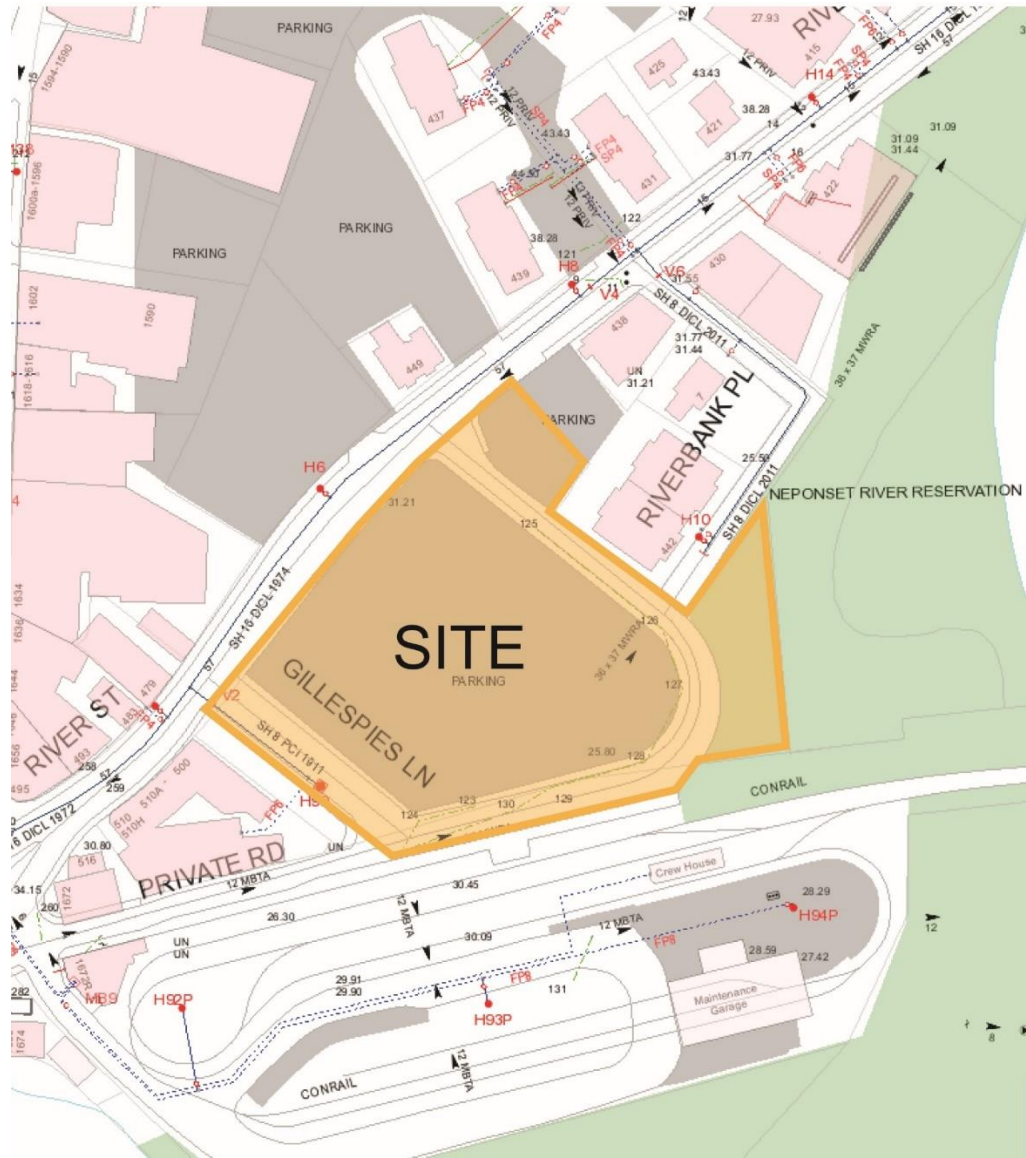
Figure 2-31 Existing Water Distribution System in the Vicinity of 466 River Street (Owned and Maintained By BWSC)
