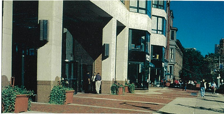
Continuity of the street wall defines lower Boylston Street. Variation is provided through the use of projecting bays as well as recessed entrances.
