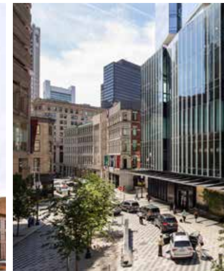
A small stepback along the front face of the Millennium Tower aligns with historic buildings along Franklin St. (Handel, Boston)
