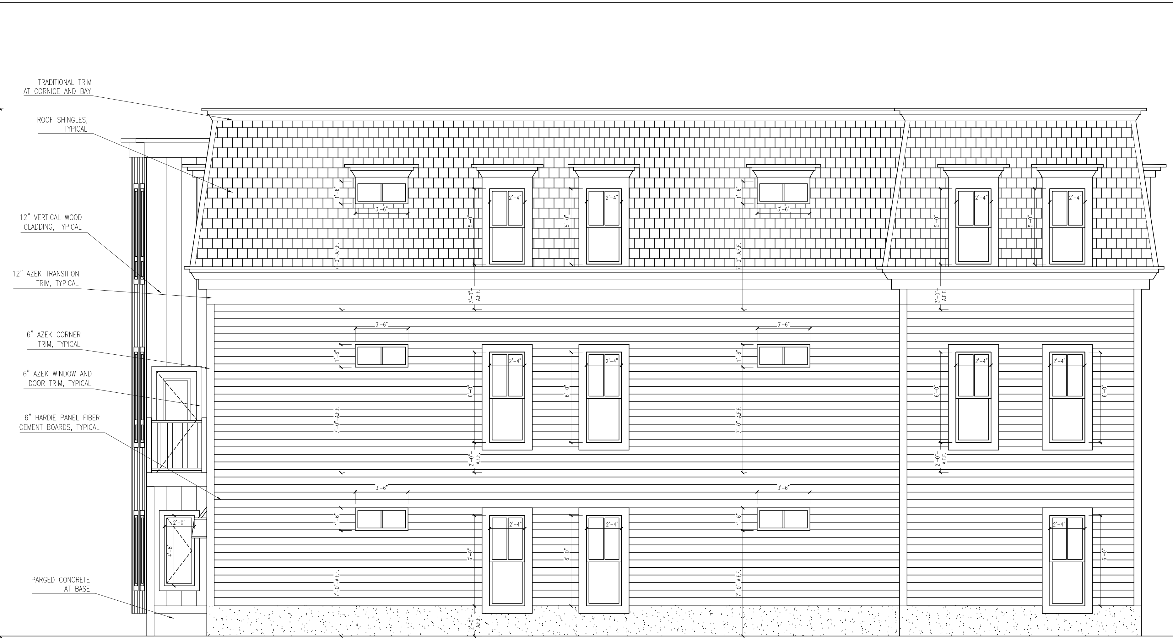
2 PROPOSED SIDE ELEVATION SCALE: 1/4" = 1'-0"
