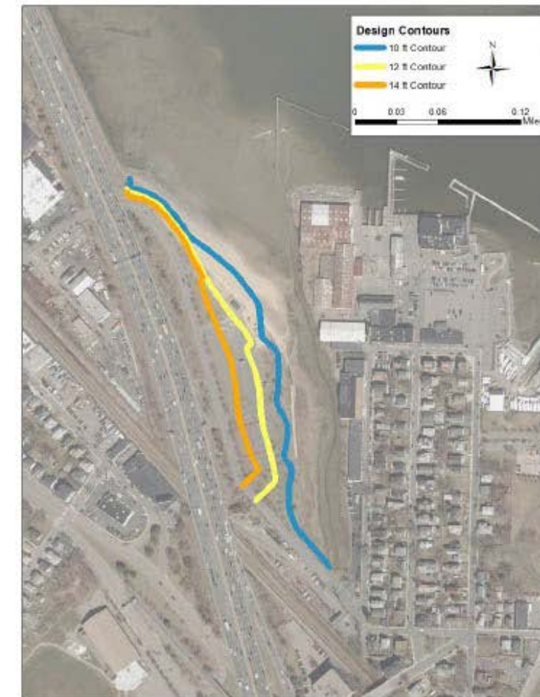
Figure 1: Approximate design alignment contours applied to the modeling domain. The design was applied to the MC-FRM modeling mesh as a series of contours representing the 10ft NAVD88 contour line, the 12 ft NAVD88 contour line, and the 14 ft NAVD88 contour line as proposed by the design drawing.
