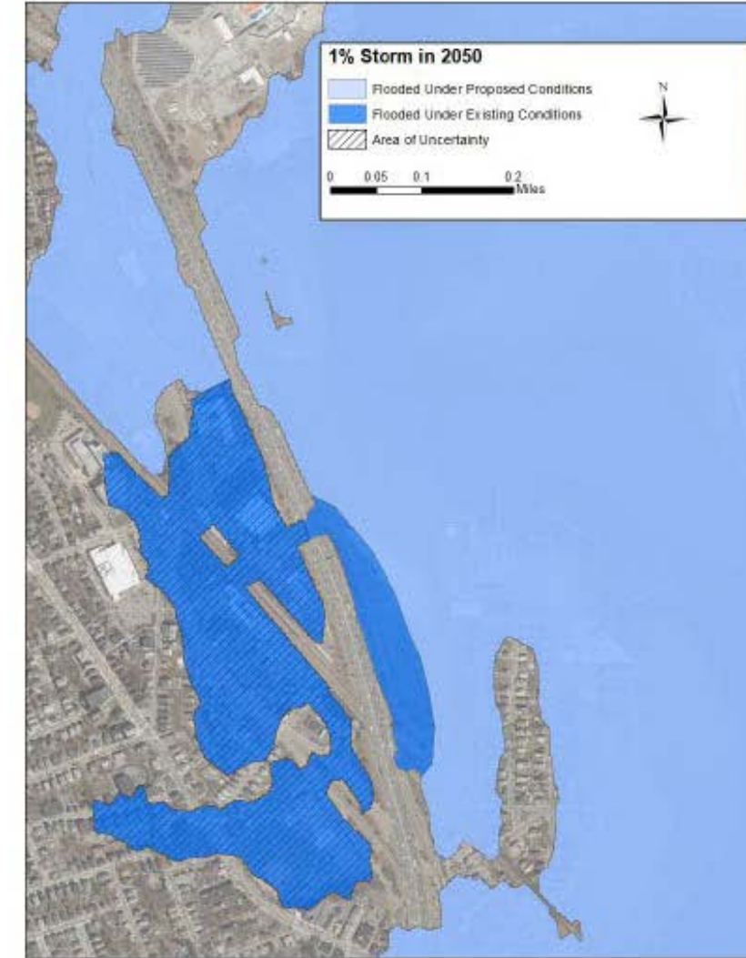
Figure 4: Flood extents for the 1% AEP storm event under the 2050 climate horizon. The light blue indicates areas that are flooded in both existing and proposed conditions, whereas the dark blue regions indicate areas of avoided flooding due to the design alternative. The hatched area represents uncertainty in the extent of flooding.
