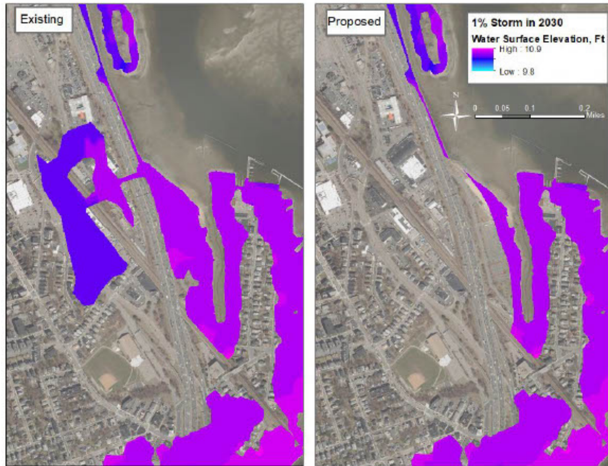
Figure 7: Water surface elevations for the 2030 1% AEP. The left panel represents existing conditions, without the project implemented, and the right panel represents proposed conditions, with the project implemented. Water surface elevations above Mean High Water (MHW) are shown in this figure, considering overland flooding only.
