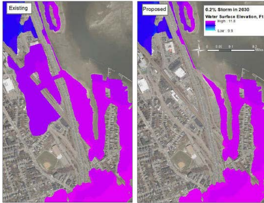
Figure 9: Water surface elevations for the 2030 0.2% AEP. The left panel represents existing conditions, without the project implemented, and the right panel represents proposed conditions, with the project implemented. Water surface elevations above MHW are shown in this figure, considering overland flooding only.
