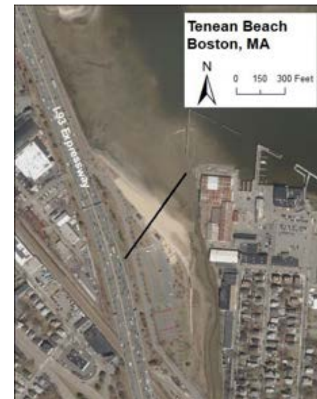
Figure 1. Xbeach 1-D cross sectional transect assessed for Tenean Beach in Boston, MA
