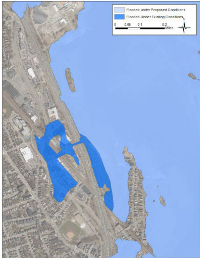
Figure 3: Flood extents for the 1% AEP storm event under the 2030 climate horizon. The light blue indicates areas that are flooded in both existing and proposed conditions, whereas the dark blue regions indicate areas of avoided flooding due to the design alternative.
