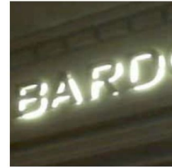
Halo Illumination Projected light from behind individual letters or symbols gives a halo effect.
