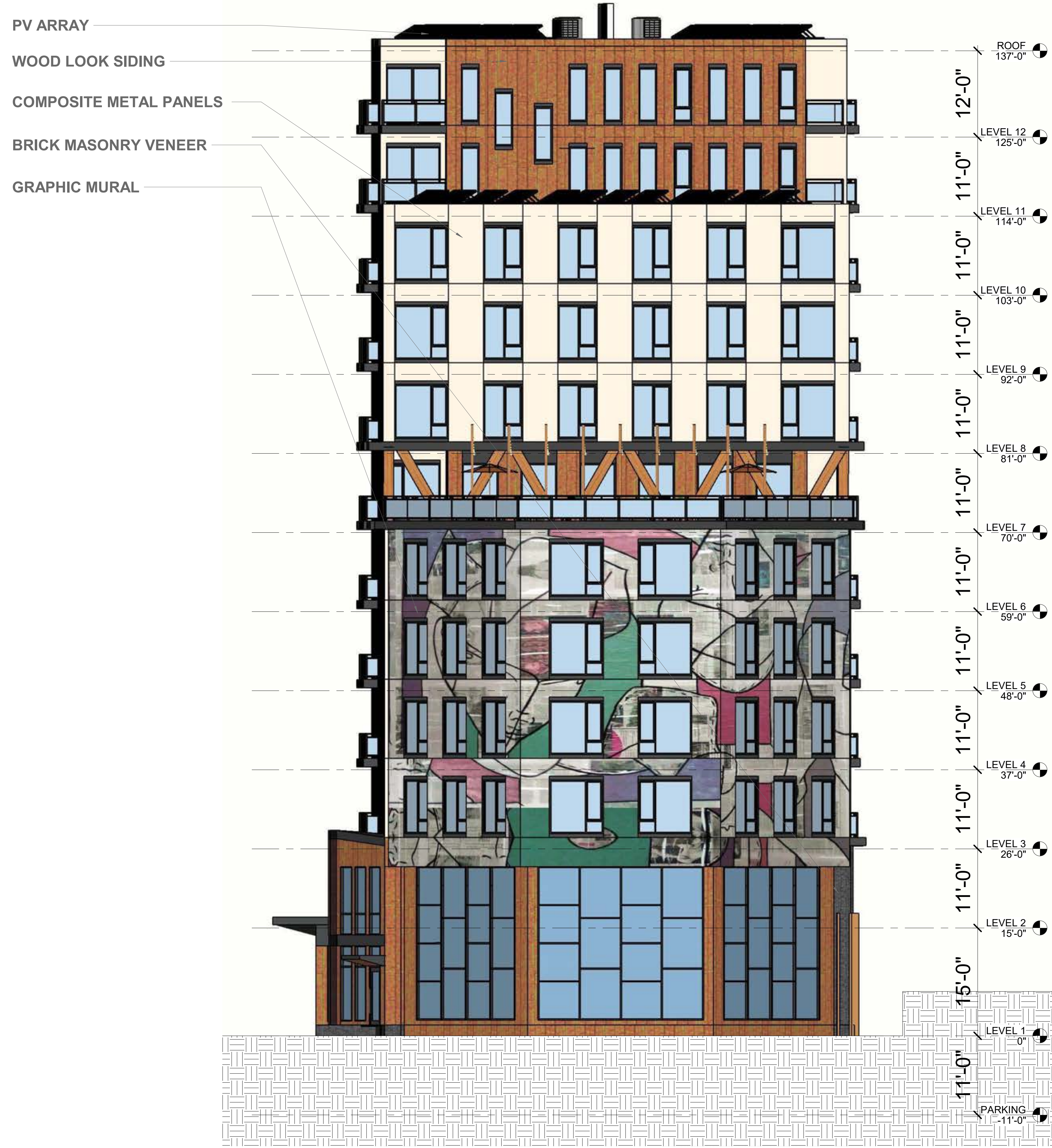
2 BUILDING 1 NORTH ELEVATION 1/8" = 1'-0"
