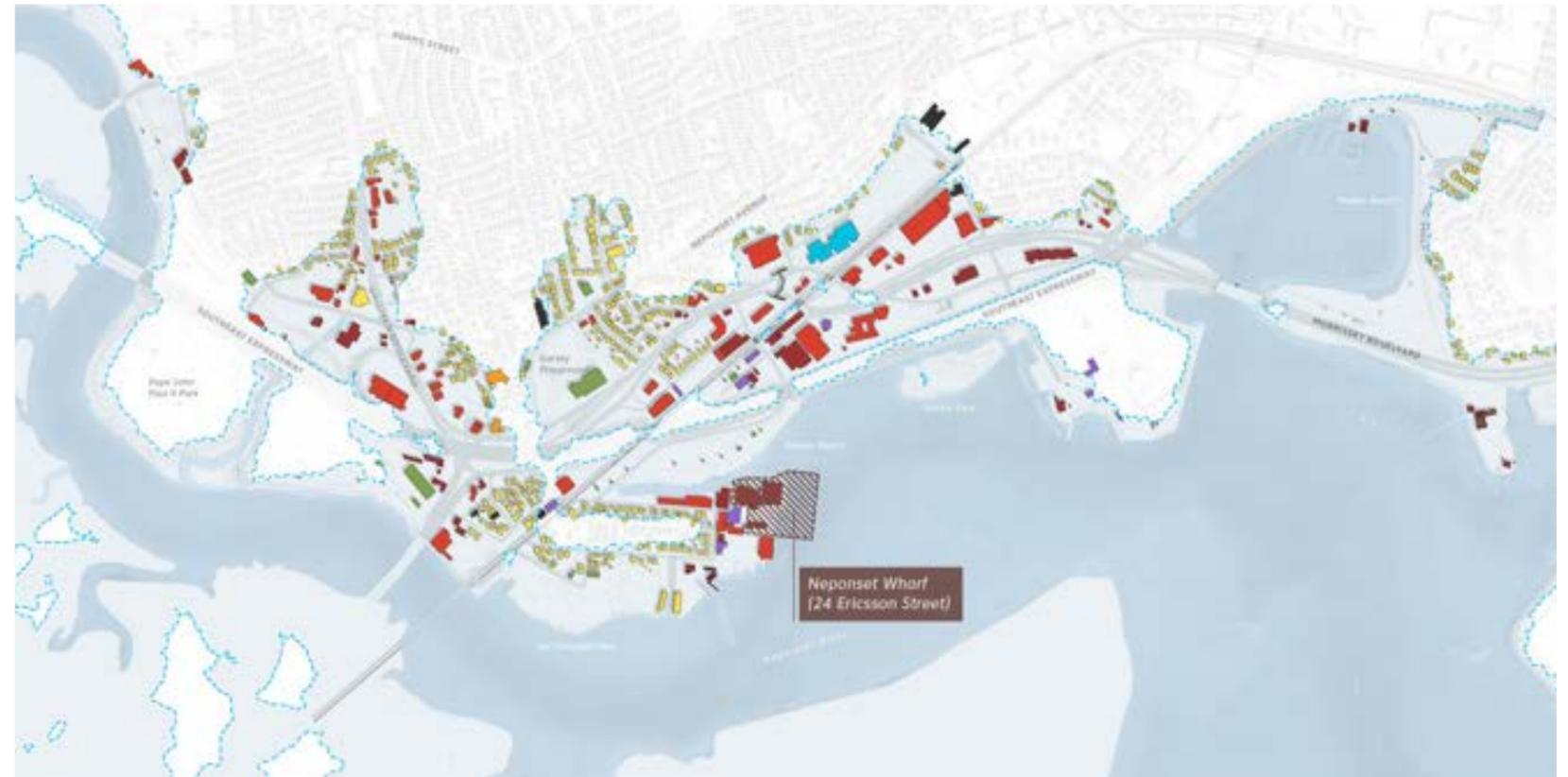
**Figure 5:** Potentially impacted buildings in a 1% Annual Chance Flood with 40 inches SLR (2070s)
